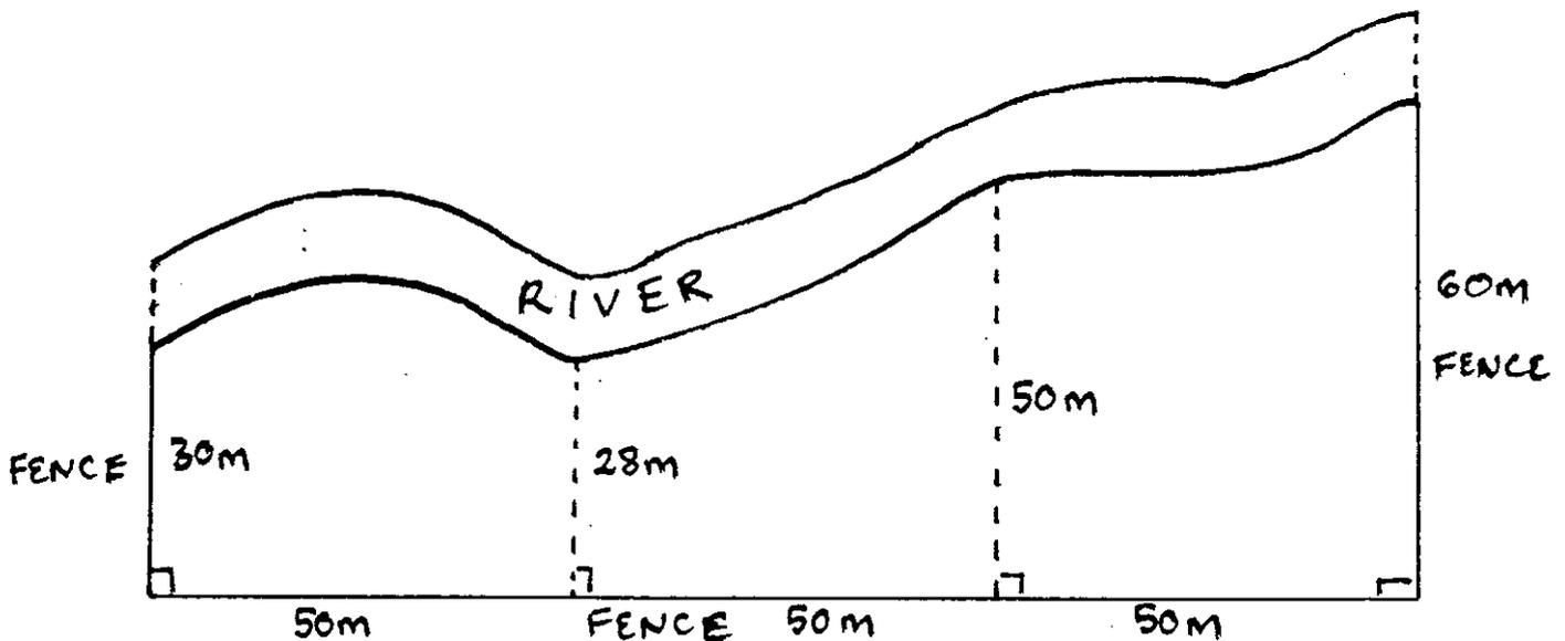
The diagram above is of a field bounded by a river and three fences. A farmer wishes to calculate the area of the field and has obtained the measurements above. Estimate the area of the field using the trapezoidal rule with four function values.
